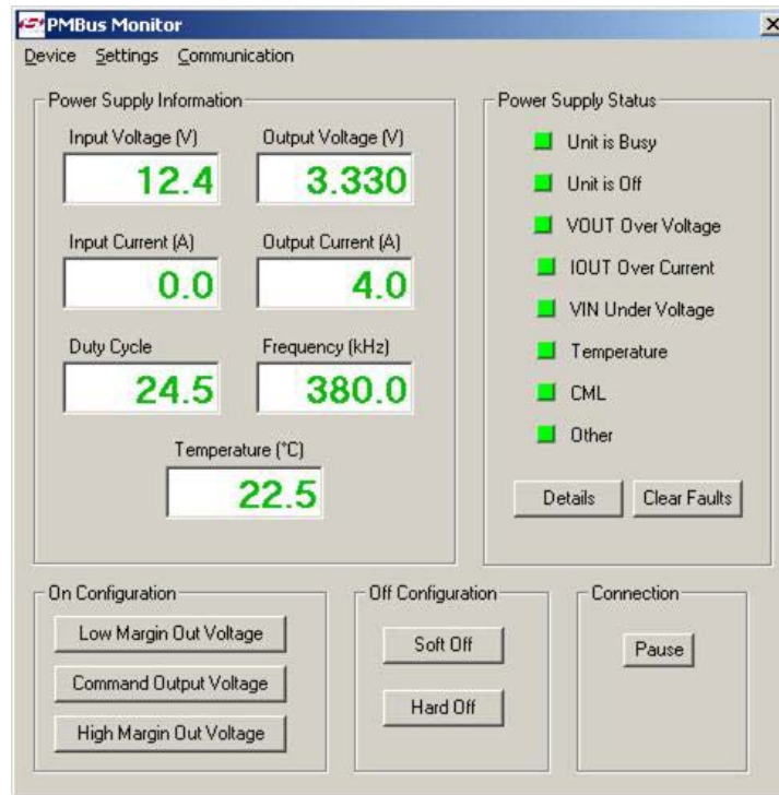
Figure 5. View of the PMBus Monitor
