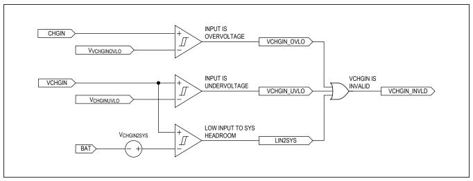
Figure 4. Charger Input Validation
