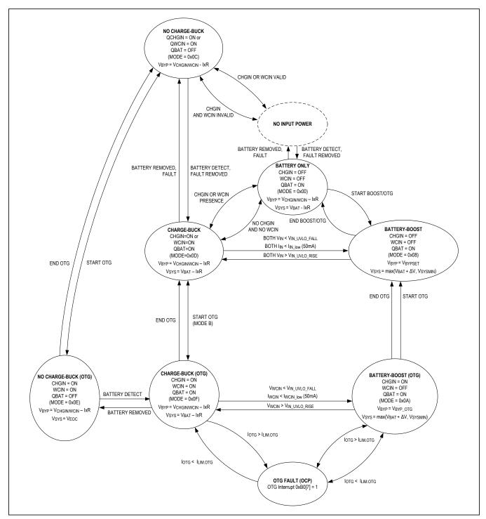
Figure 9: Power State Diagram
