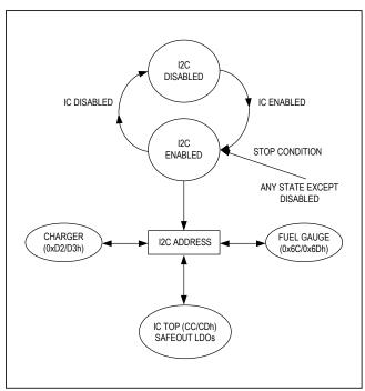
Figure 17. I<sup>2</sup>C Slave Address Structure
