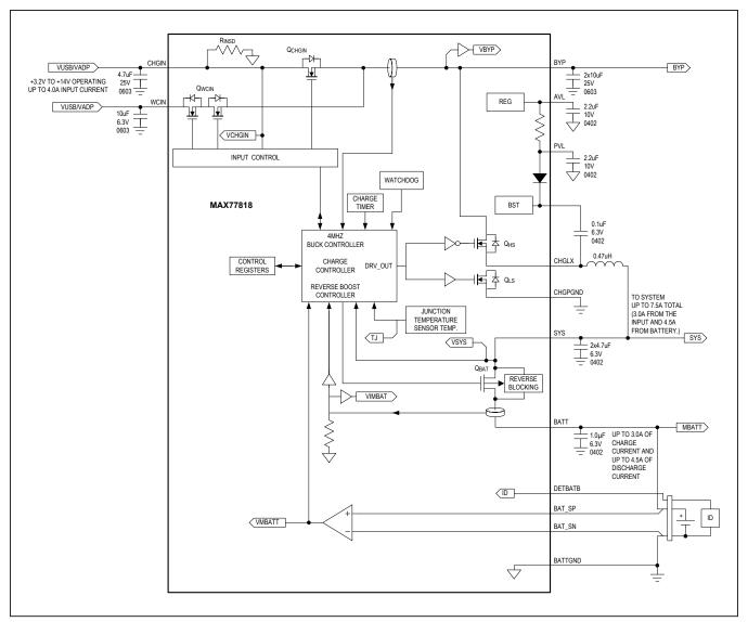
Figure 2. Main Battery Charger Detailed Functional Diagram
