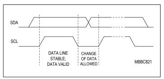
Figure 18. I<sup>2</sup>C Bit Transfer
