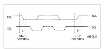
Figure 19. I<sup>2</sup>C Start and Stop
