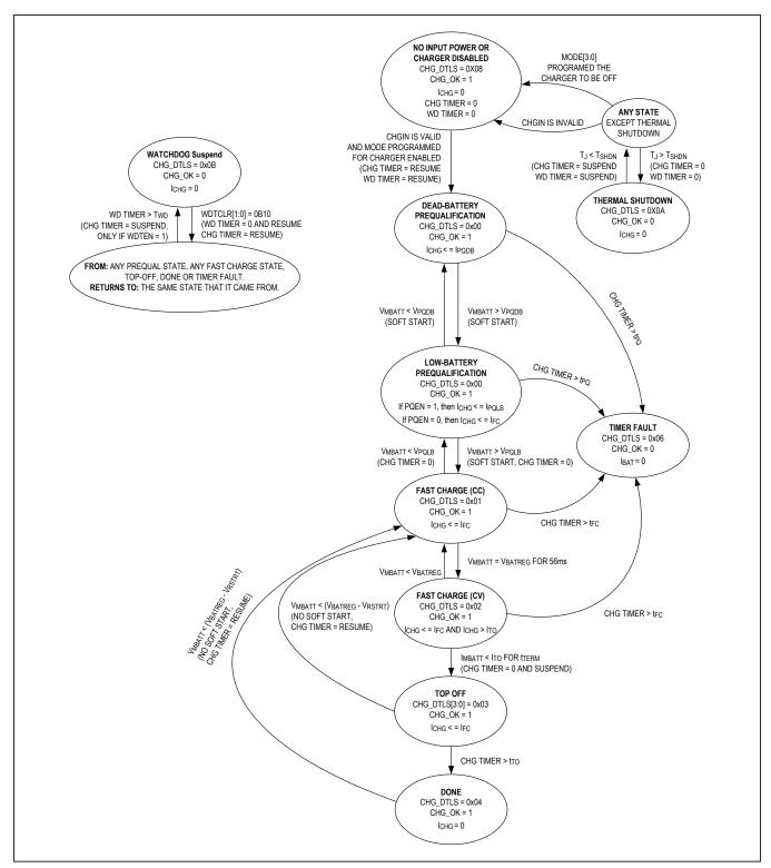
Figure 7. Charger State Diagram
