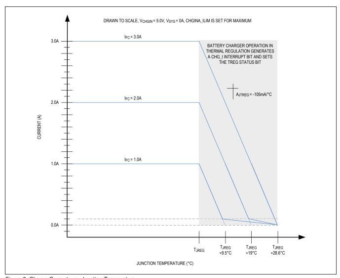
Figure 8. Charge Currents vs. Junction Temperature
