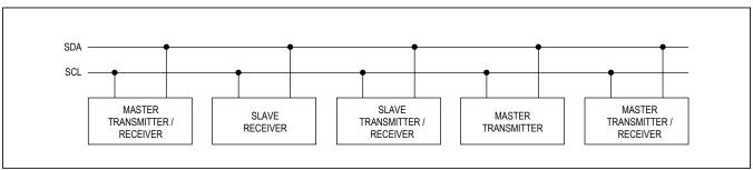
Figure 20. I<sup>2</sup>C System Configuration
