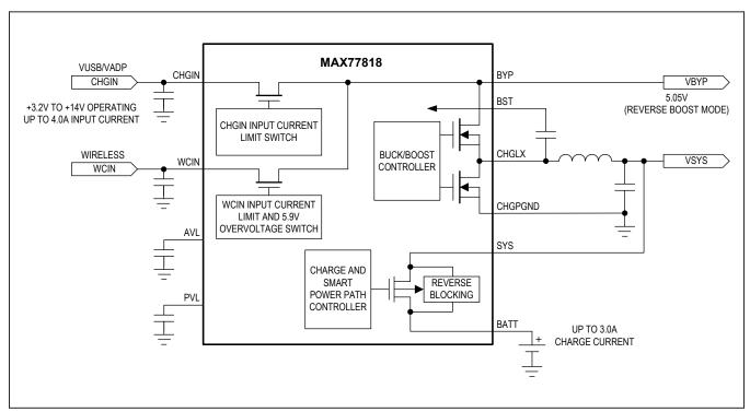
Figure 1. Simplified Functional Diagram
