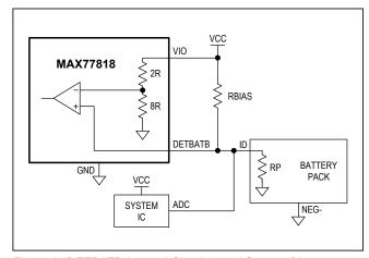
Figure 3. DETBATB Internal Circuitry and System Diagram
