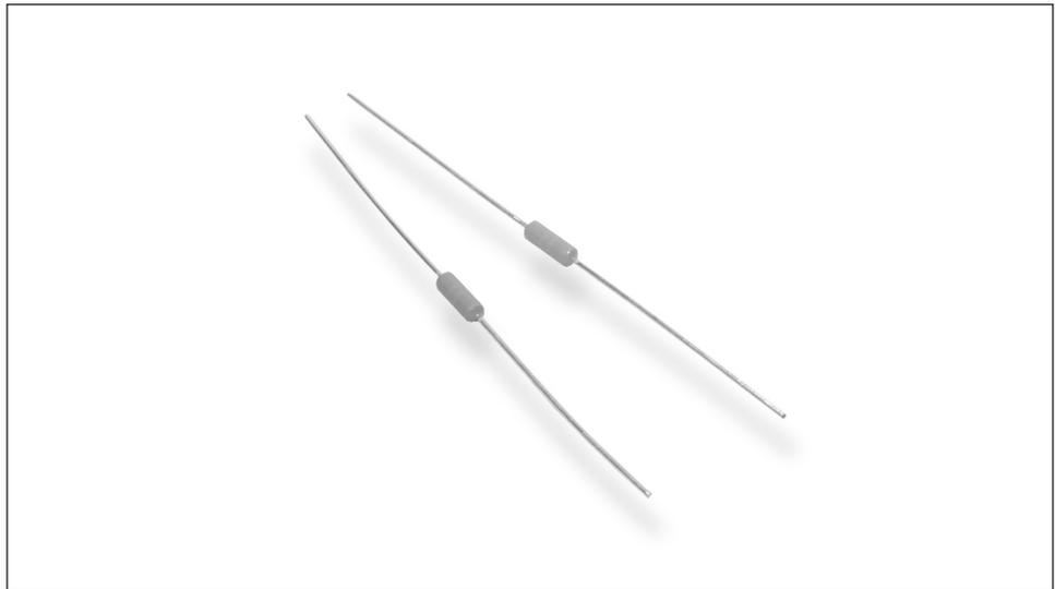
The TE Connectivity Series of Zerohm links are available in two standard case sizes and element types. No end caps are used for the steel element, terminations are welded directly on to the steel slug. For the Ceramic elements, tinned copper wire leads are welded onto end caps. This manufacturing process allows for very low resistance values to be achieved. The slugs are then finished by applying three coats of light brown epoxy resin.
