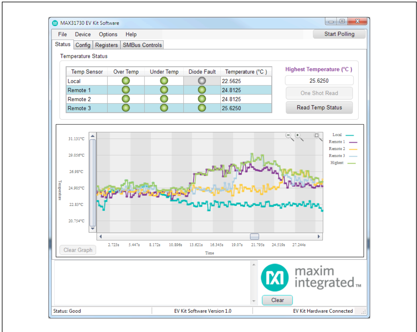
Figure 1. MAX31730 EV Kit Software GUI (Status Tab)
