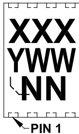
14-Lead SOIC (150 mil) (MCP6444)
