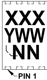
14-Lead SOIC (150 mil) (MCP6444)
