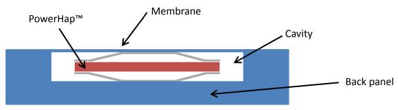
In this case the PowerHap actuator is clamped between a thin, flexible membrane and a rigid back panel. By applying a voltage, the actuator elongates and consequently deforms the membrane.
