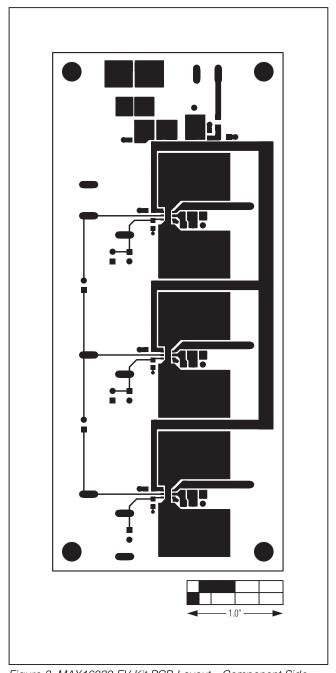
Figure 3. MAX16839 EV Kit PCB Layout—Component Side
