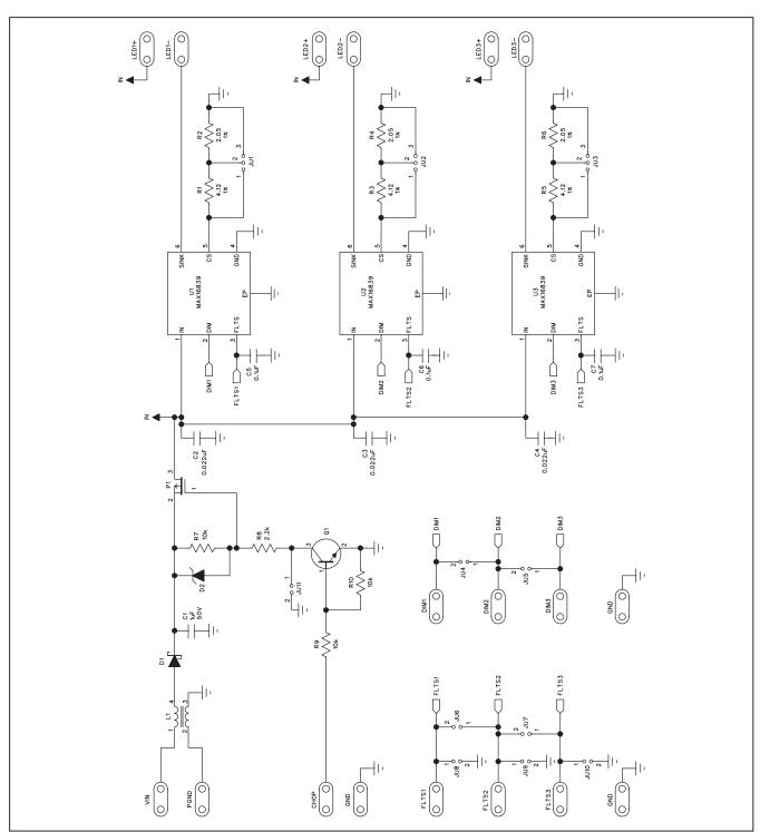
Figure 1. MAX16839 EV Kit Schematic
