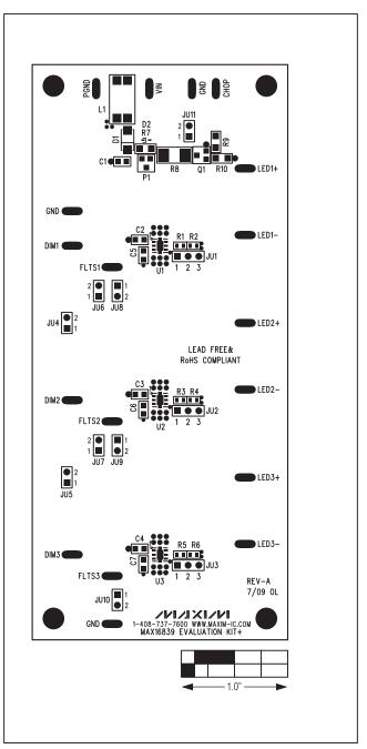
Figure 2. MAX16839 EV Kit Component Placement Guide—Component Side
