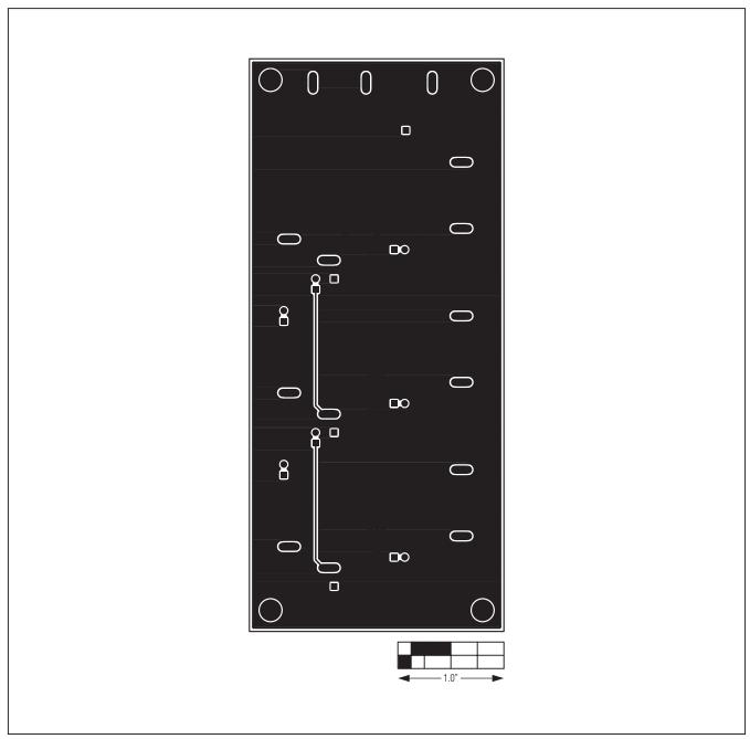
Figure 4. MAX16839 EV Kit PCB Layout—Solder Side
