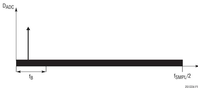
Figure 15. Frequency Spectrum of SAR ADC Core Output
