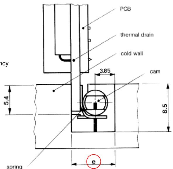
This measure does not take into account the convection and the radiation phenomena, but allows the determination of the thermal resistance of the clamp coupling, for which the values are dependant on the length of the thermal clamp.
