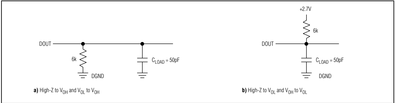
Figure 1. Load Circuits for DOUT Enable Time
