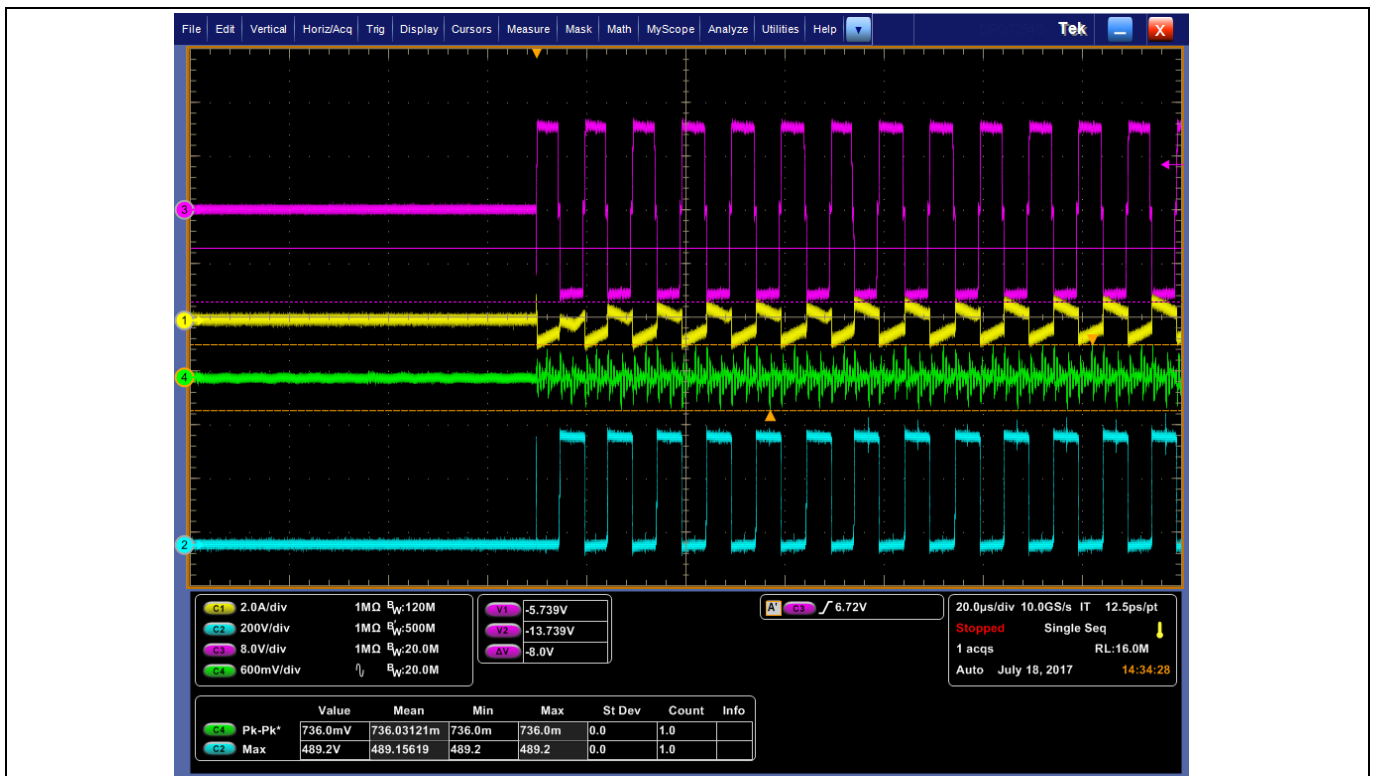
Figure 42 Burst ripple: output voltage (green), primary current (yellow), V GS of bridge low-side MOSFET (purple) and V DS of bridge low-side MOSFET (blue)
