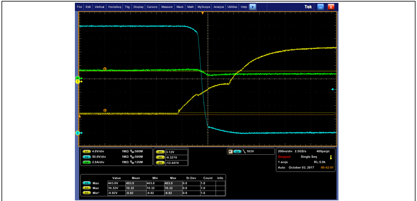
Figure 62 Lagging leg achieves ZVS at I_{out} = 24 A. Waveforms captured on MOSFET D: V_{ds} (blue); V_{gs} (yellow); primary current (green).
