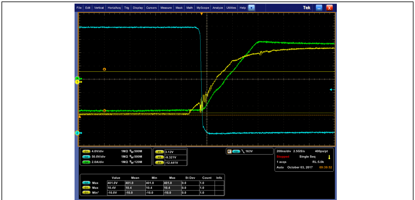
Figure 63 Leading leg achieves ZVS at 117 A. Waveforms captured on MOSFET B: V_{DS} (blue); V_{GS} (yellow); primary current (green).
