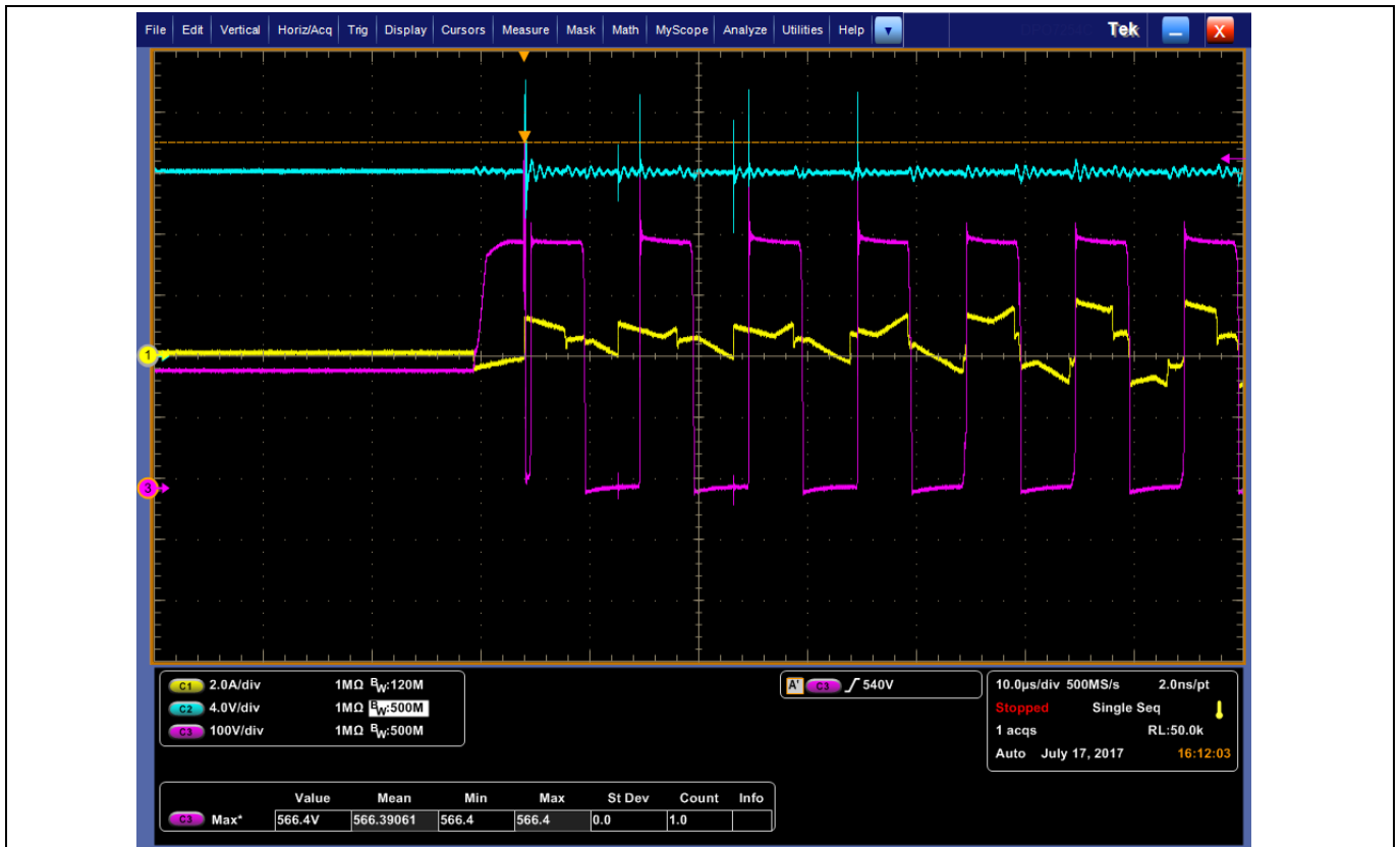
Figure 69 Short-circuit under no load at output. Primary current (yellow), output voltage (blue), MOSFET V_{DS} (purple).
