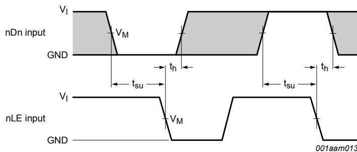
**Fig. 8. Data setup and hold times for input (nDn) to input (nLE)**
