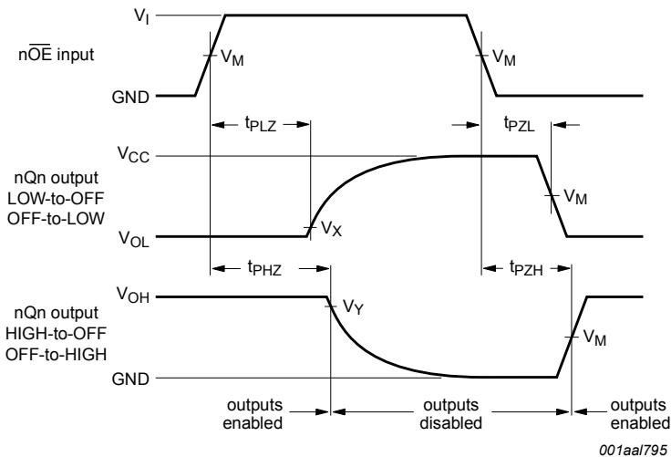
**Fig. 9. 3-State enable and disable times**
