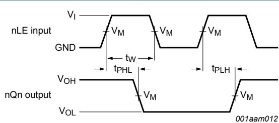
**Fig. 7. Latch enable input (nLE) to data output (nQn) propagation delays and pulse width (nLE)**
