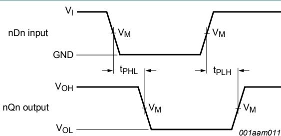
**Fig. 6. Input (nDn) to output (nQn) propagation delays**
