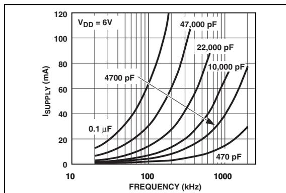
**FIGURE 2-12:** Supply Current vs. Frequency ( $V_{DD} = 6\text{V}$ ).
