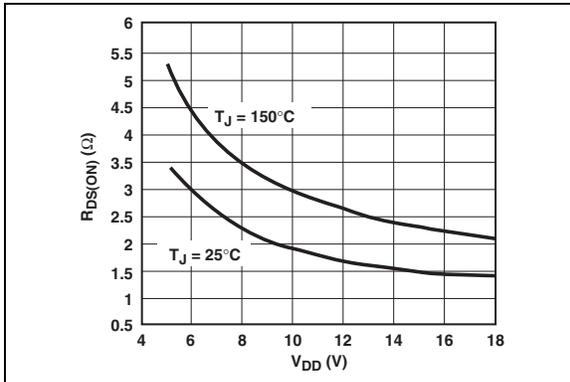
**FIGURE 2-15:** High-State Output Resistance vs. Supply Voltage.
