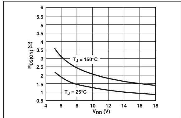
**FIGURE 2-18:** Low-State Output Resistance vs. Supply Voltage.
