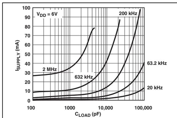
**FIGURE 2-9:** Supply Current vs. Capacitive Load ( $V_{DD} = 6\text{V}$ ).
