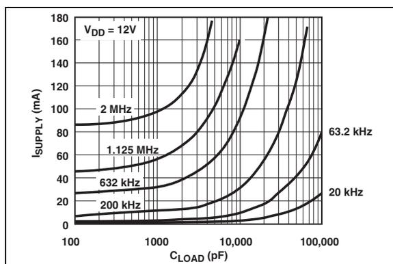
**FIGURE 2-8:** Supply Current vs. Capacitive Load ( $V_{DD} = 12\text{V}$ ).
