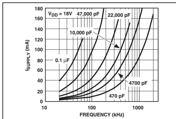
**FIGURE 2-10:** Supply Current vs. Frequency ( $V_{DD} = 18\text{V}$ ).
