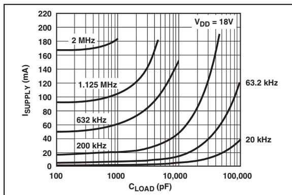
**FIGURE 2-7:** Supply Current vs. Capacitive Load ( $V_{DD} = 18\text{V}$ ).
