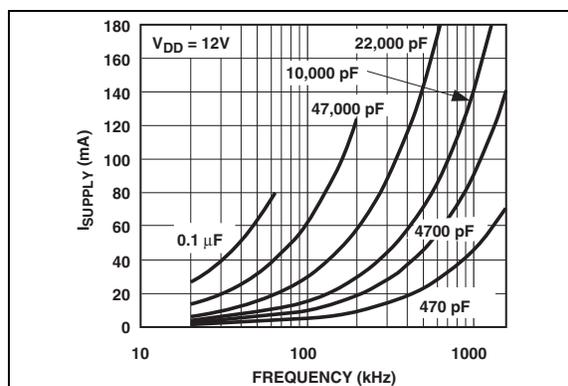
**FIGURE 2-11:** Supply Current vs. Frequency ( $V_{DD} = 12\text{V}$ ).
