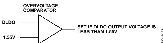
Figure 121. Digital LDO Monitor
