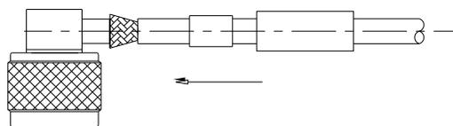
7. CRIMP OUTER FERRULE WITH APPROPRIATE CRIMP TOOL.
