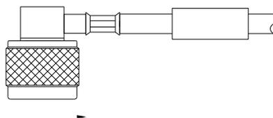
8. SLIDE AND SCREW NUT. SLIDE SHRINK TUBING OVER CRIMP AND SHRINK
