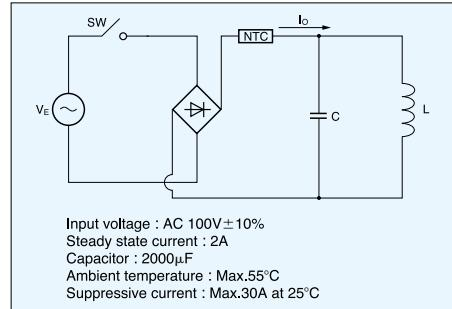
The most suitable power thermistor for the above circuit is required to fulfill the following terms and conditions.
