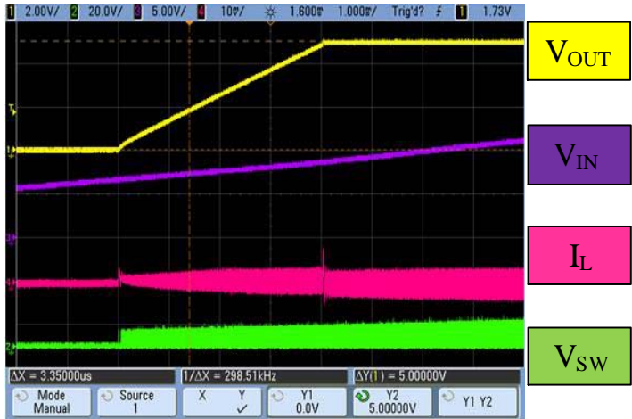
Figure 21. Start-Up Transition at No Load
