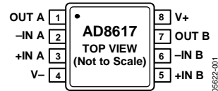
Figure 2. 8-Lead MSOP and 8-Lead SOIC_N
