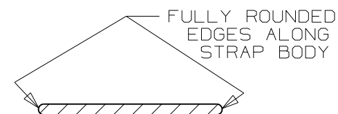
SECTION A - A SCALE 8 : 1
