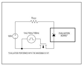
Figure 1. MAX5991A/MAX5991B Internal TVS Test Setup
