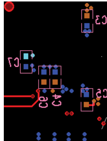
Figure 42. Bottom Layer Decoupling
