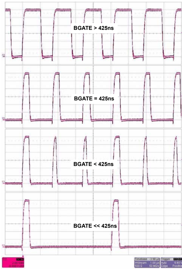
FIGURE 4. BGATE PULSE STRETCHING
