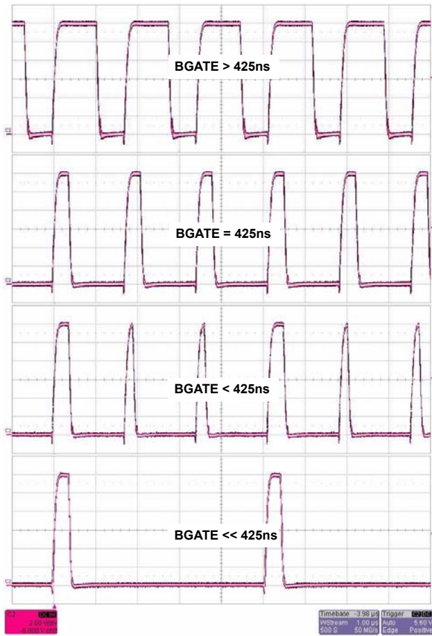
FIGURE 4. BGATE PULSE STRETCHING
