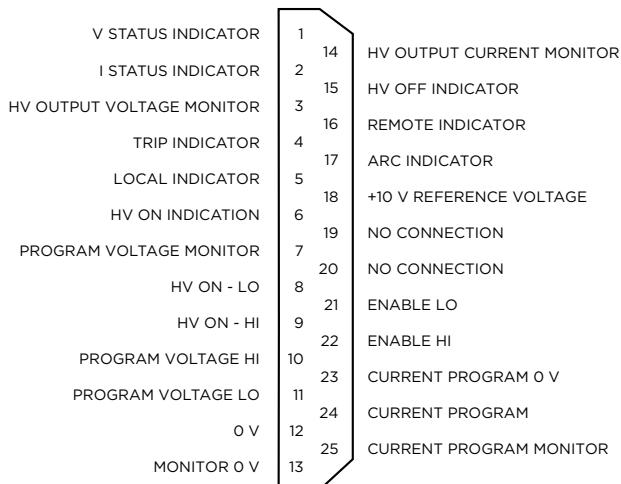
All logical indicators are open collector outputs rated at 16 V (max) in the OFF state. An internal 100 Ω resistor is connected in series with the open collector transistor. The pull down voltage is 0.9 V plus the internal resistor drop. The rated current is 10 mA.
