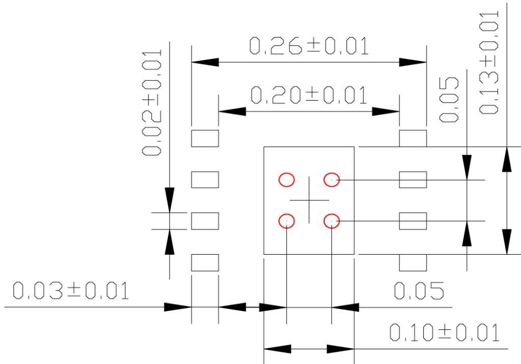
**Red circle** indicates Thermal Via. Size should be .015-.017 inches in diameter and it should be connected to GND plane for maximum thermal performance.
