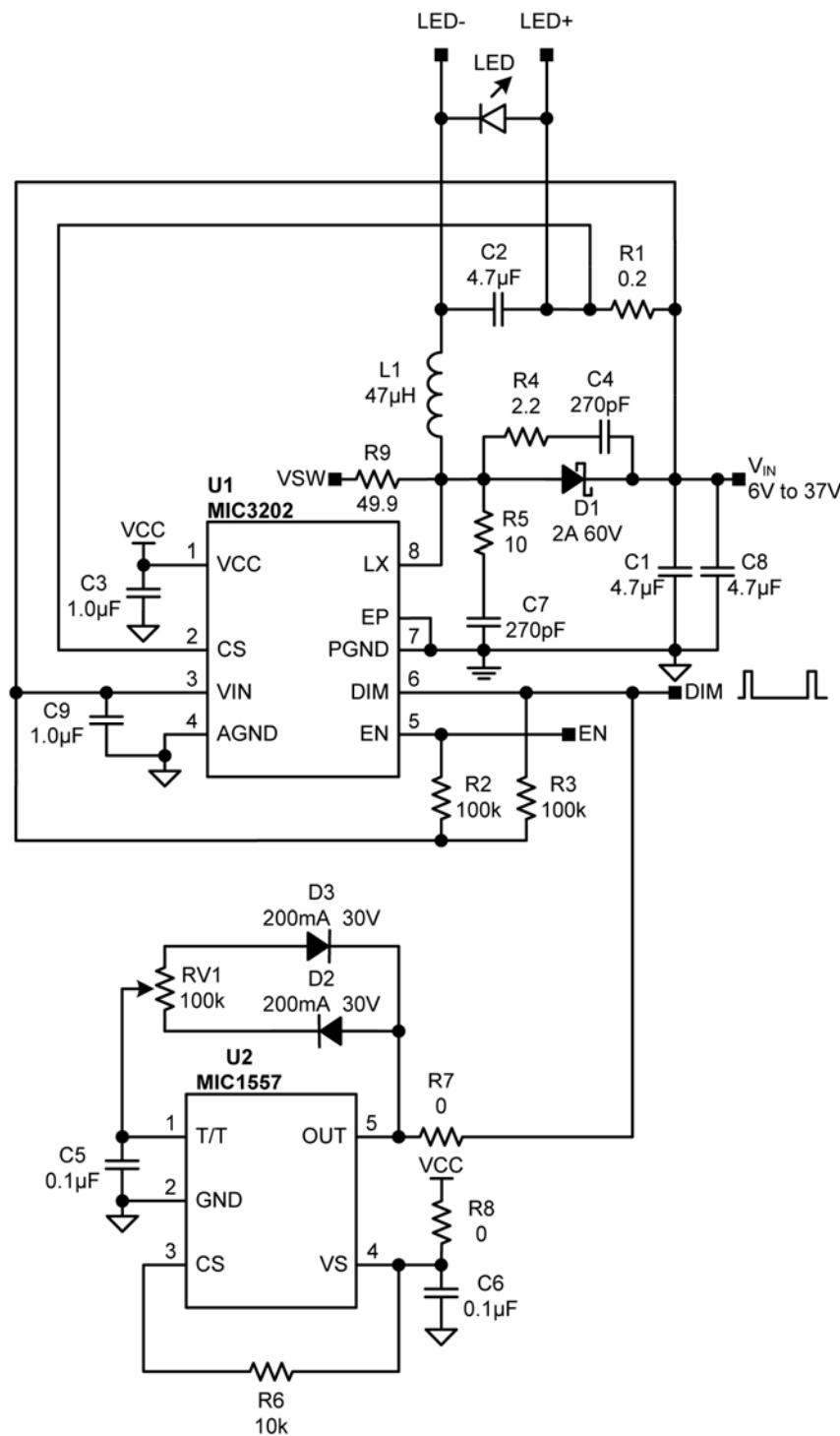
**Figure 3. MIC3202 Application Circuit
