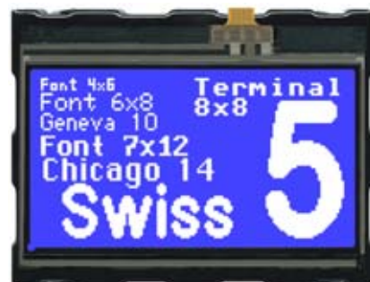
integrated fonts in delivery state
