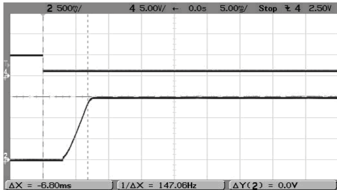
Step Load Transient Response (Vin=12V, Vout=1.5V, Cload=0, Iout=8A to 16A) Trace 2=Vout, 100 mV/div., Trace4=Iout, 5A/div.
