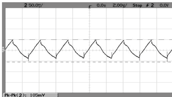
Output Ripple and Noise (V IN =12V, V OUT =5V, I OUT =16A, C LOAD =0, ScopeBW=100MHz)
