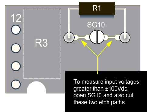
Figure 4. Installing R1
