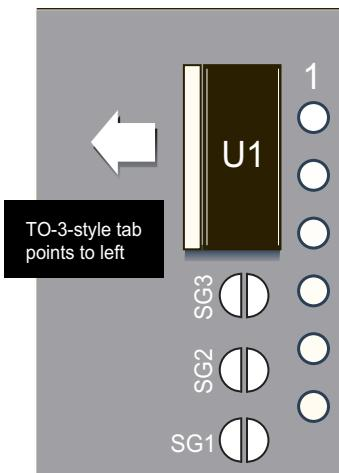
Figure 3. Installing U1
