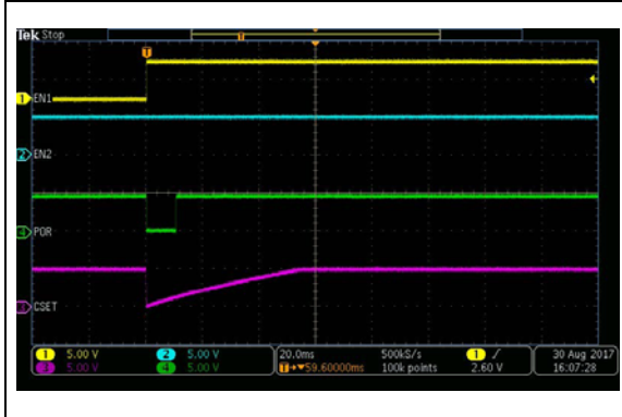
FIGURE 2-37: POR Behavior, EN2 = High, Low-to-High Transition on EN1.
