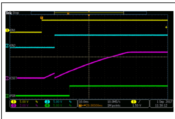
FIGURE 2-38: CSET Pin Voltage and POR Delay Time Behavior for Correct Sequencing.
