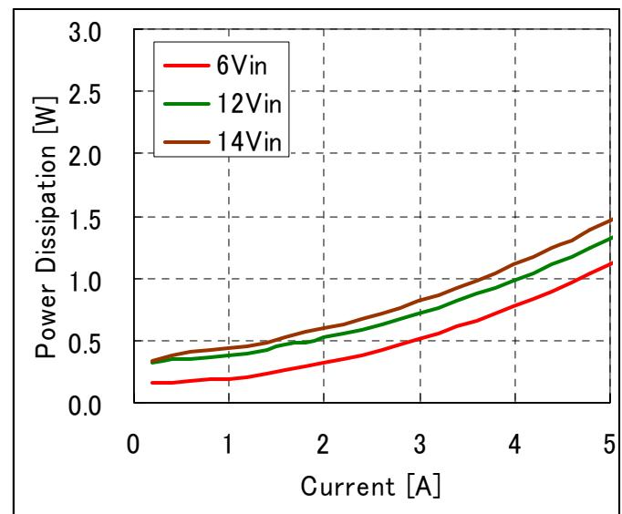
**Fig-1.8V-3:** Power Loss vs. load current and input voltage for  $V_{out}=1.8V$ .
