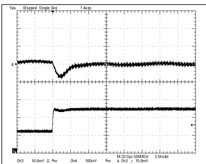
**Fig-1.0V-6:** Output voltage response for  $V_{out}=1.0V$  to positive load current step change from 2.5A to 5A with slew rate of  $5A/\mu s$  at  $V_{in}=12V$ .  $C_o=47\mu Fx2$  ceramic.
