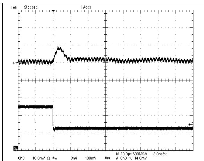
**Fig-3.3V-7:** Output voltage response for  $V_{out}=3.3V$  to negative load current step change from 5A to 2.5A with slew rate of -5A/ $\mu s$  at  $V_{in}=12V$ .  $C_o=47\mu Fx2$  ceramic.
