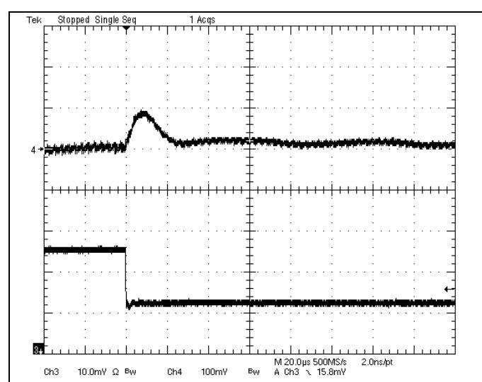
**Fig-1.2V-7:** Output voltage response for  $V_{out}=1.2V$  to negative load current step change from 5A to 2.5A with slew rate of -5A/us at  $V_{in}=12V$ .  $C_o=47\mu Fx2$  ceramic.
