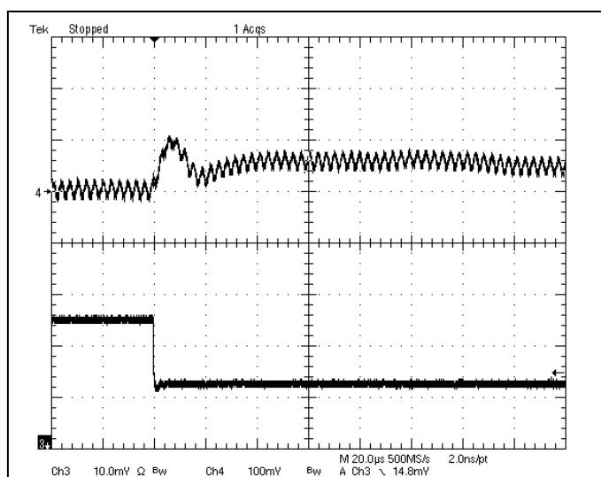
**Fig-5.0V-7:** Output voltage response for  $V_{out}=5.0V$  to negative load current step change from 5A to 2.5A with slew rate of  $-5A/\mu s$  at  $V_{in}=12V$ .  $C_o=47\mu Fx2$  ceramic.
