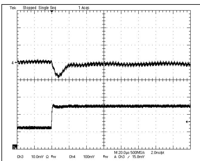
**Fig-2.0V-6:** Output voltage response for  $V_{out}=2.0V$  to positive load current step change from 2.5A to 5A with slew rate of  $5A/\mu s$  at  $V_{in}=12V$ .  $C_o=47\mu Fx2$  ceramic.
