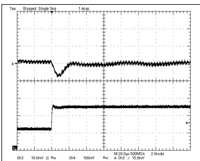
**Fig-1.8V-6:** Output voltage response for  $V_{out}=1.8V$  to positive load current step change from 2.5A to 5A with slew rate of  $5A/\mu s$  at  $V_{in}=12V$ .  $C_o=47\mu Fx2$  ceramic.
