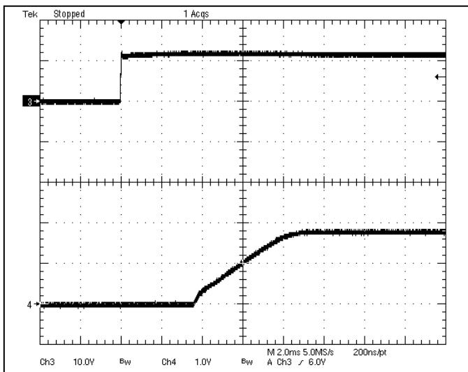
**Fig-1.8V-4:** Turn-on transient for  $V_{out}=1.8V$  with application of  $V_{in}$  at full rated load current (resistive) and  $47\mu Fx2$  external capacitance at  $V_{in}=12V$ .
