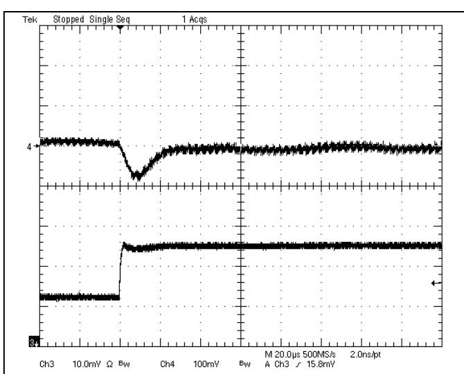
**Fig-1.2V-6:** Output voltage response for  $V_{out}=1.2V$  to positive load current step change from 2.5A to 5A with slew rate of 5A/us at  $V_{in}=12V$ .  $C_o=47\mu Fx2$  ceramic.
