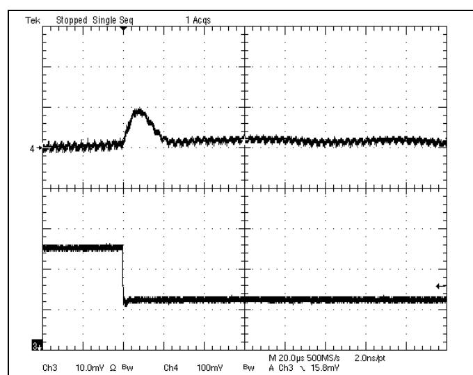
**Fig-1.8V-7:** Output voltage response for  $V_{out}=1.8V$  to negative load current step change from 5A to 2.5A with slew rate of  $-5A/\mu s$  at  $V_{in}=12V$ .  $C_o=47\mu Fx2$  ceramic.
