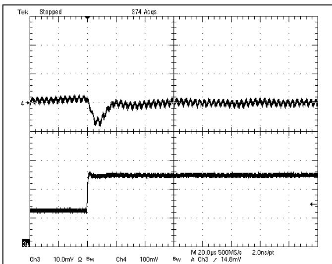
**Fig-3.3V-6:** Output voltage response for  $V_{out}=3.3V$  to positive load current step change from 2.5A to 5A with slew rate of 5A/ $\mu s$  at  $V_{in}=12V$ .  $C_o=47\mu Fx2$  ceramic.
