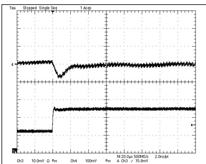
**Fig-1.5V-6:** Output voltage response for  $V_{out}=1.5V$  to positive load current step change from 2.5A to 5A with slew rate of  $5A/\mu s$  at  $V_{in}=12V$ .  $C_o=47\mu Fx2$  ceramic.
