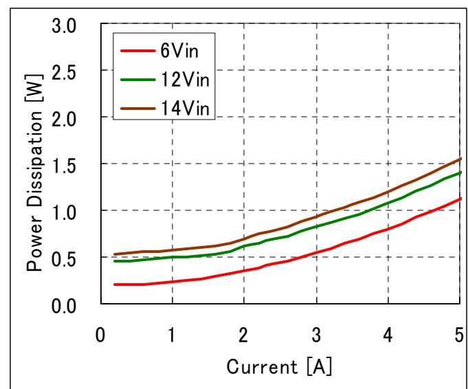
**Fig-2.5V-3:** Power Loss vs. load current and input voltage for  $V_{out}=2.5V$ .
