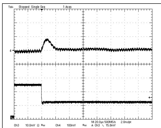
**Fig-2.0V-7:** Output voltage response for  $V_{out}=2.0V$  to negative load current step change from 5A to 2.5A with slew rate of  $-5A/\mu s$  at  $V_{in}=12V$ .  $C_o=47\mu Fx2$  ceramic.
