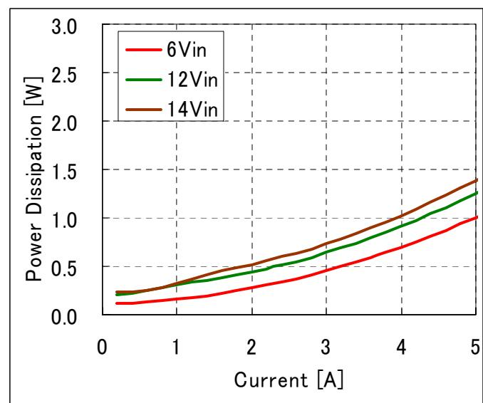
**Fig-1.2V-3:** Power Loss vs. load current and input voltage for  $V_{out}=1.2V$ .
