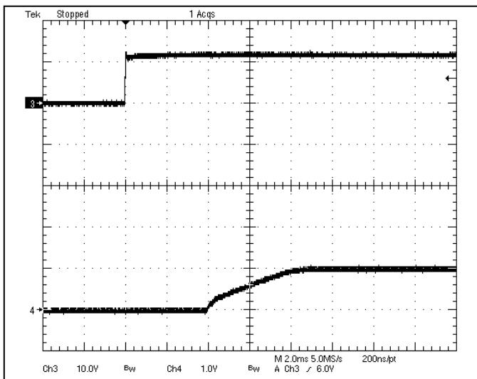
**Fig-1.0V-4:** Turn-on transient for  $V_{out}=1.0V$  with application of  $V_{in}$  at full rated load current (resistive) and  $47\mu Fx2$  external capacitance at  $V_{in}=12V$ .
