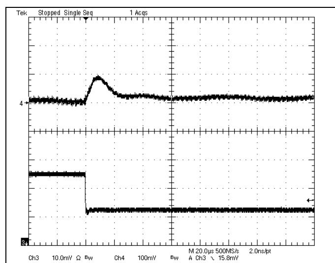
**Fig-1.0V-7:** Output voltage response for  $V_{out}=1.0V$  to negative load current step change from 5A to 2.5A with slew rate of  $-5A/\mu s$  at  $V_{in}=12V$ .  $C_o=47\mu Fx2$  ceramic.
