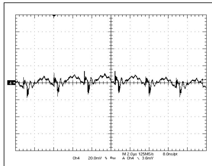
**Fig-1.2V-5:** Output voltage ripple (20mV/div.) for  $V_{out}=1.2V$  at full rated load current into a resistive load with external capacitance  $47\mu Fx2$  ceramic +  $1\mu F$  ceramic at  $V_{in}=12V$ .
