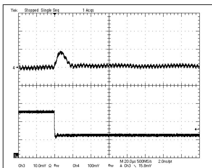
**Fig-2.5V-7:** Output voltage response for  $V_{out}=2.5V$  to negative load current step change from 5A to 2.5A with slew rate of  $-5A/\mu s$  at  $V_{in}=12V$ .  $C_o=47\mu Fx2$  ceramic.
