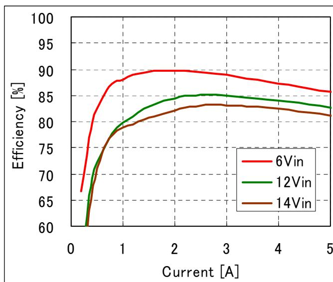
**Fig-1.2V-2:** Efficiency vs. load current and input voltage for  $V_{out}=1.2V$ .
