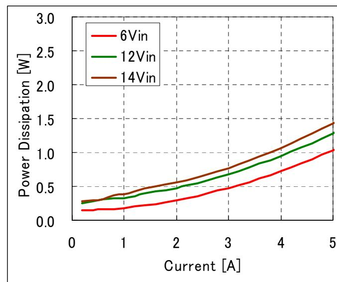
**Fig-1.5V-3:** Power Loss vs. load current and input voltage for  $V_{out}=1.5V$ .
