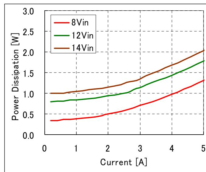
**Fig-5.0V-3:** Power Loss vs. load current and input voltage for  $V_{out}=5.0V$ .
