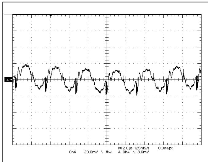
**Fig-5.0V-5:** Output voltage ripple (20mV/div.) for  $V_{out}=5.0V$  at full rated load current into a resistive load with external capacitance  $47\mu Fx2$  ceramic +  $1\mu F$  ceramic at  $V_{in}=12V$ .
