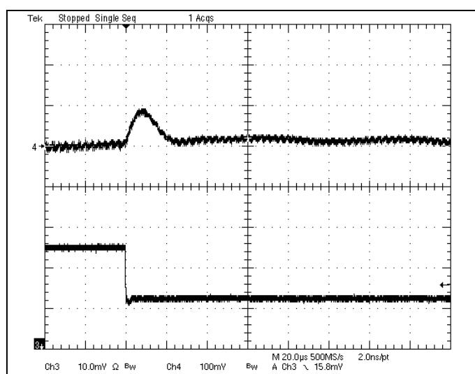
**Fig-1.5V-7:** Output voltage response for  $V_{out}=1.5V$  to negative load current step change from 5A to 2.5A with slew rate of  $-5A/\mu s$  at  $V_{in}=12V$ .  $C_o=47\mu Fx2$  ceramic.
