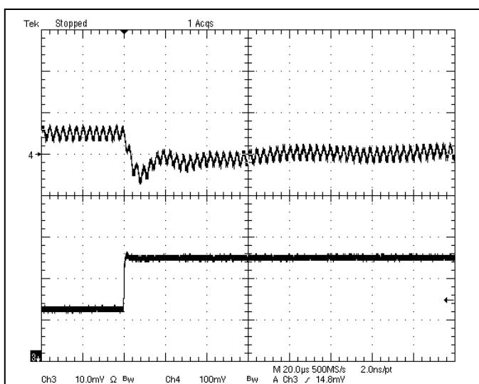
**Fig-5.0V-6:** Output voltage response for  $V_{out}=5.0V$  to positive load current step change from 2.5A to 5A with slew rate of  $5A/\mu s$  at  $V_{in}=12V$ .  $C_o=47\mu Fx2$  ceramic.
