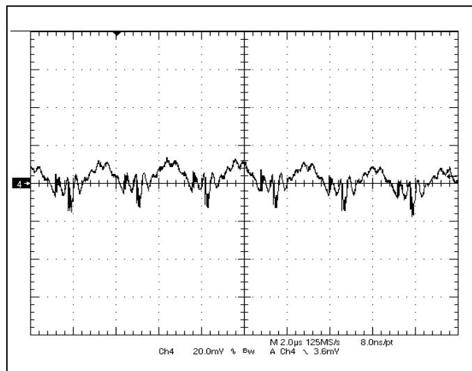
**Fig-2.0V-5:** Output voltage ripple (20mV/div.) for  $V_{out}=2.0V$  at full rated load current into a resistive load with external capacitance  $47\mu Fx2$  ceramic +  $1\mu F$  ceramic at  $V_{in}=12V$ .
