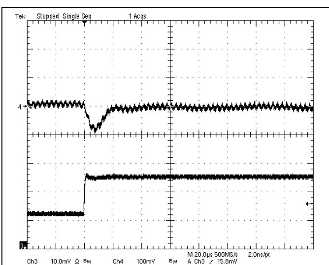
**Fig-2.5V-6:** Output voltage response for  $V_{out}=2.5V$  to positive load current step change from 2.5A to 5A with slew rate of  $5A/\mu s$  at  $V_{in}=12V$ .  $C_o=47\mu Fx2$  ceramic.
