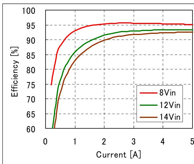
**Fig-5.0V-2:** Efficiency vs. load current and input voltage for  $V_{out}=5.0V$ .
