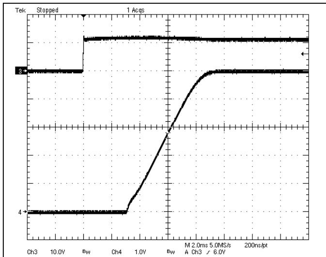
**Fig-5.0V-4:** Turn-on transient for  $V_{out}=5.0V$  with application of  $V_{in}$  at full rated load current (resistive) and  $47\mu Fx2$  external capacitance at  $V_{in}=12V$ .
