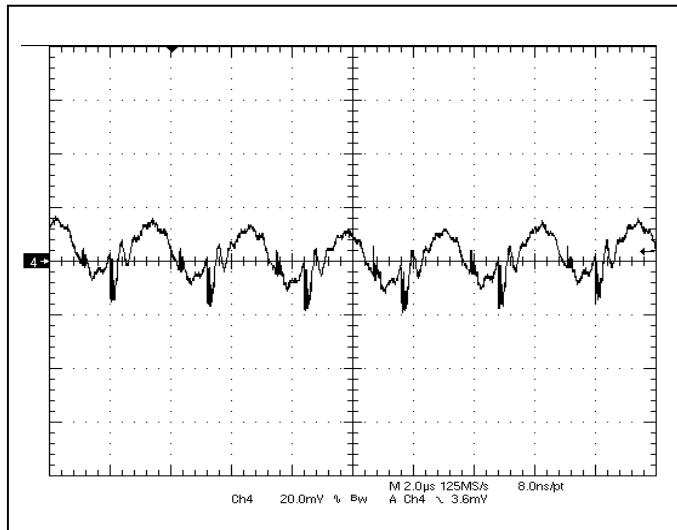
**Fig-3.3V-5:** Output voltage ripple (20mV/div.) for  $V_{out}=3.3V$  at full rated load current into a resistive load with external capacitance  $47\mu Fx2$  ceramic +  $1\mu F$  ceramic at  $V_{in}=12V$ .
