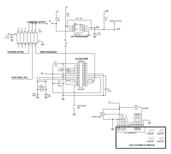
Figure 16. Evaluation Board Schematic (2 of 2)
