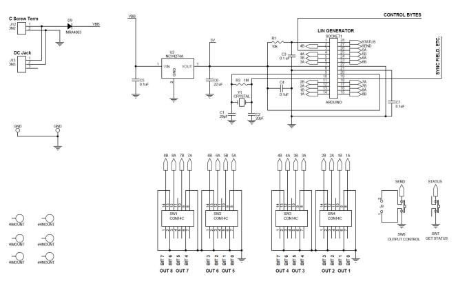
Figure 15. Evaluation Board Schematic (1 of 2)
