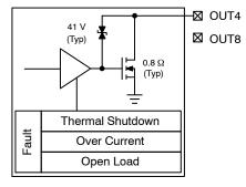
Figure 3. 0.8  $\Omega$  Output Drivers
