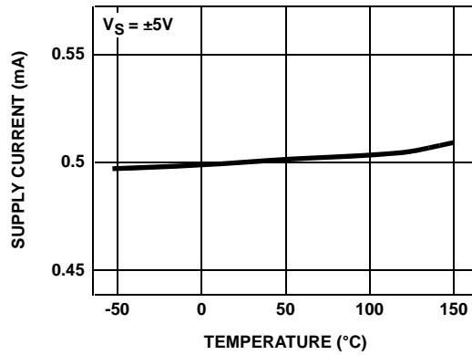
FIGURE 9. EL5420 SUPPLY CURRENT PER AMPLIFIER vs TEMPERATURE
