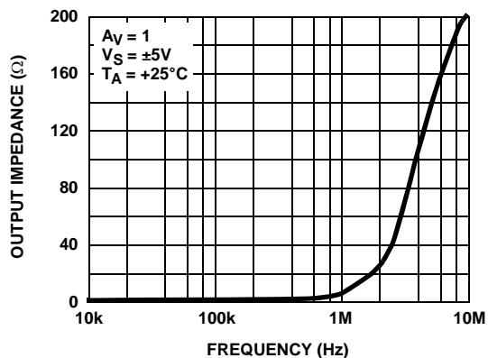
FIGURE 14. CLOSED LOOP OUTPUT IMPEDANCE vs FREQUENCY
