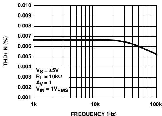
FIGURE 19. TOTAL HARMONIC DISTORTION + NOISE vs FREQUENCY
