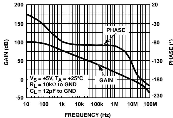
FIGURE 11. OPEN LOOP GAIN AND PHASE vs FREQUENCY
