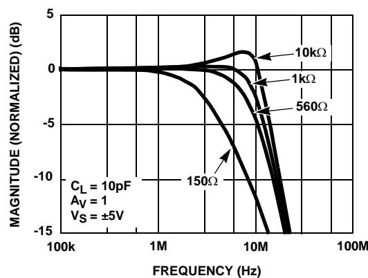
FIGURE 12. FREQUENCY RESPONSE FOR VARIOUS R<sub>L</sub>
