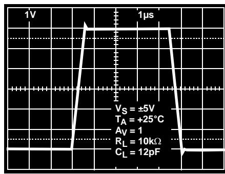
FIGURE 23. LARGE SIGNAL TRANSIENT RESPONSE
