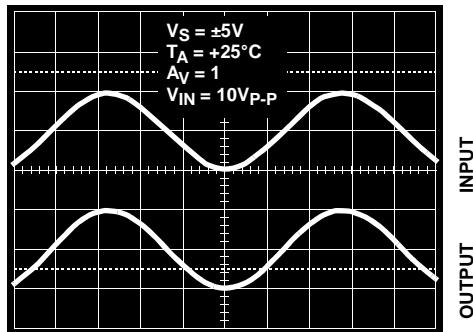
**FIGURE 25. OPERATION WITH RAIL-TO-RAIL INPUT AND OUTPUT**
