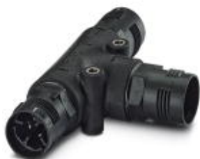
T distributor, QUICKON connection, number of positions: 4+PE, 1 mm 2 ... 2.5 mm 2 , 690 V, 20 A, black, Without QUICKON nut
