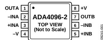
Figure 1. 8-Lead, MSOP (RM-8), ADA4096-2
