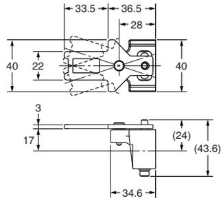
**Note:** Unless otherwise specified, a tolerance of  $\pm 0.8$  mm applies to all Switch dimensions and a tolerance of  $\pm 0.4$  mm applies to Operation Key dimensions.
