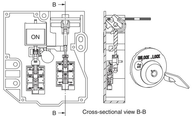
**(3) Operation Key inserted, solenoid OFF, and trapped key inserted. Status: Door locked and trapped key cannot be removed.**
