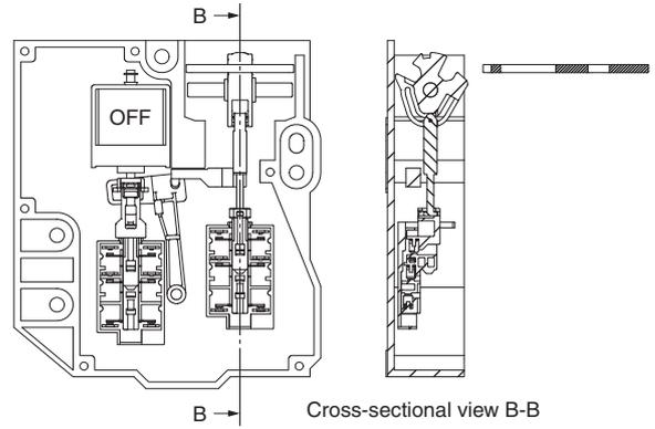
Operation Key inserted: Door unlocked.
