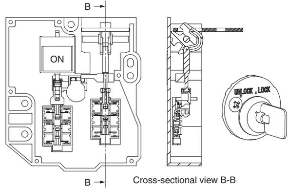
**(2) Operation Key inserted, solenoid OFF, and trapped key removed. Status: Door unlocked.**
