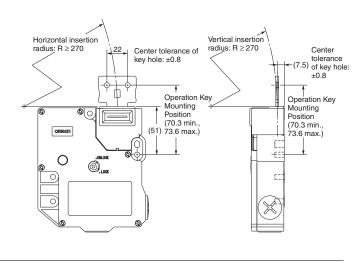
D4JL+D4JL-K2 (with Front-inserted Operation Key)
