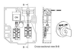
(2) Operation Key inserted, solenoid OFF, and trapped key removed. Status: Door unlocked.
