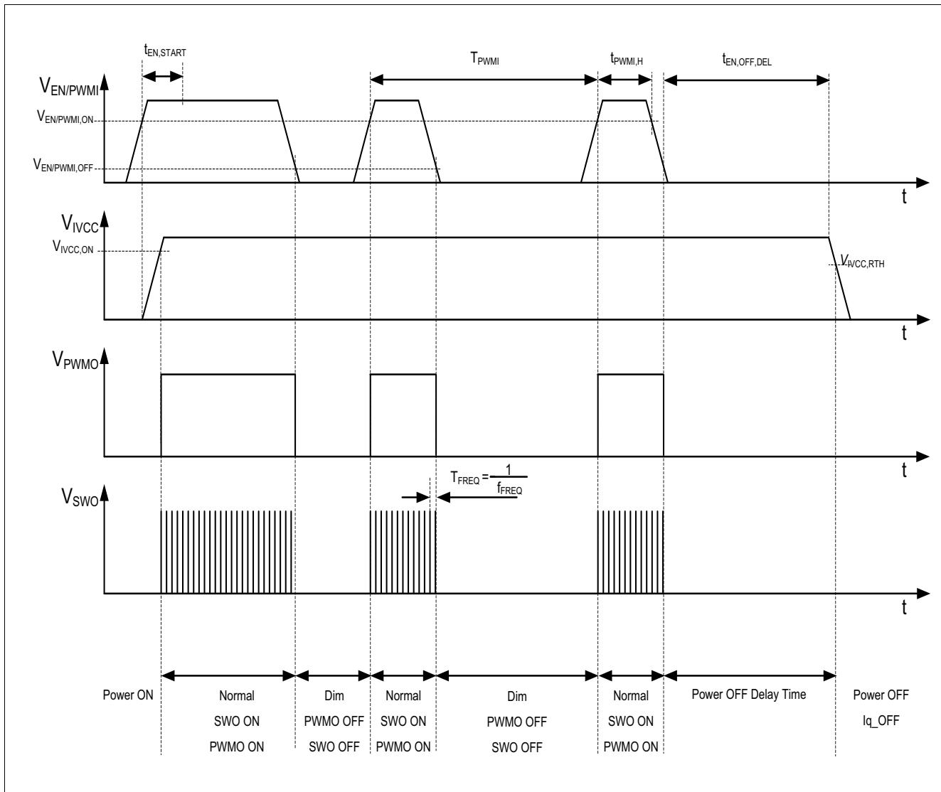
Figure 7 Timing Diagram Enable and LED Dimming
