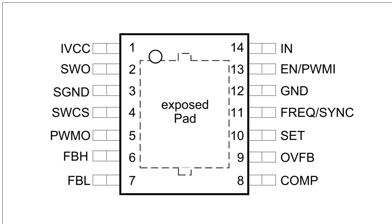
Figure 2 Pin Configuration
