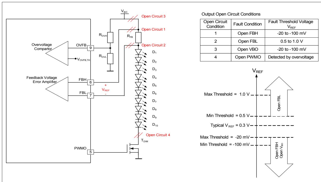
Figure 11 Open Load and Open Feedback Conditions
