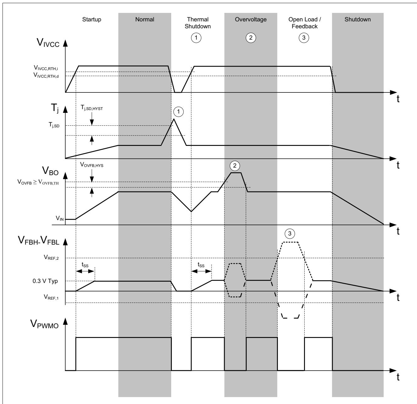
Figure 12 Open load, Overvoltage and Overtemperature Timing Diagram
