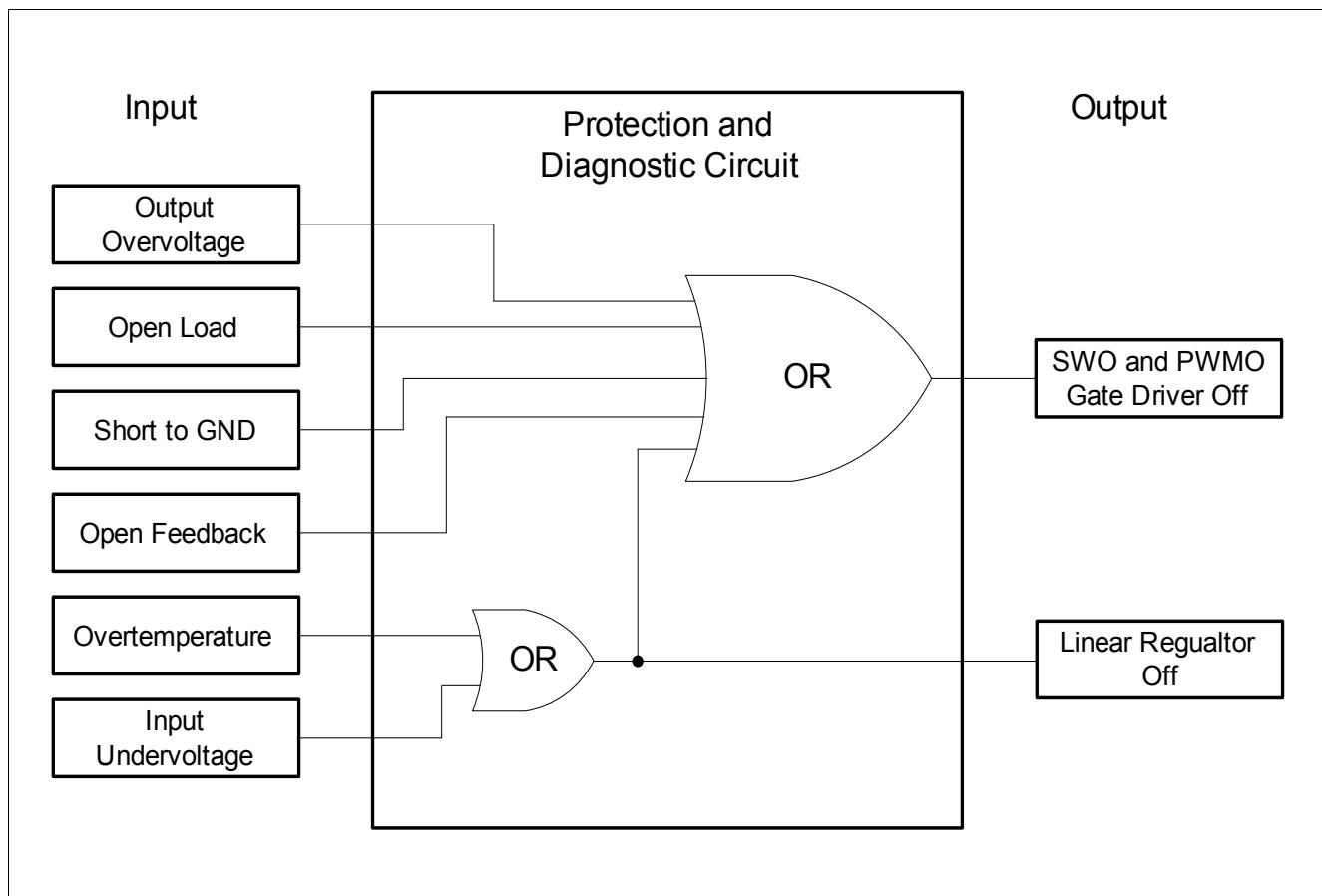
**Figure 9 Protection and Diagnostic Function Block Diagram**
