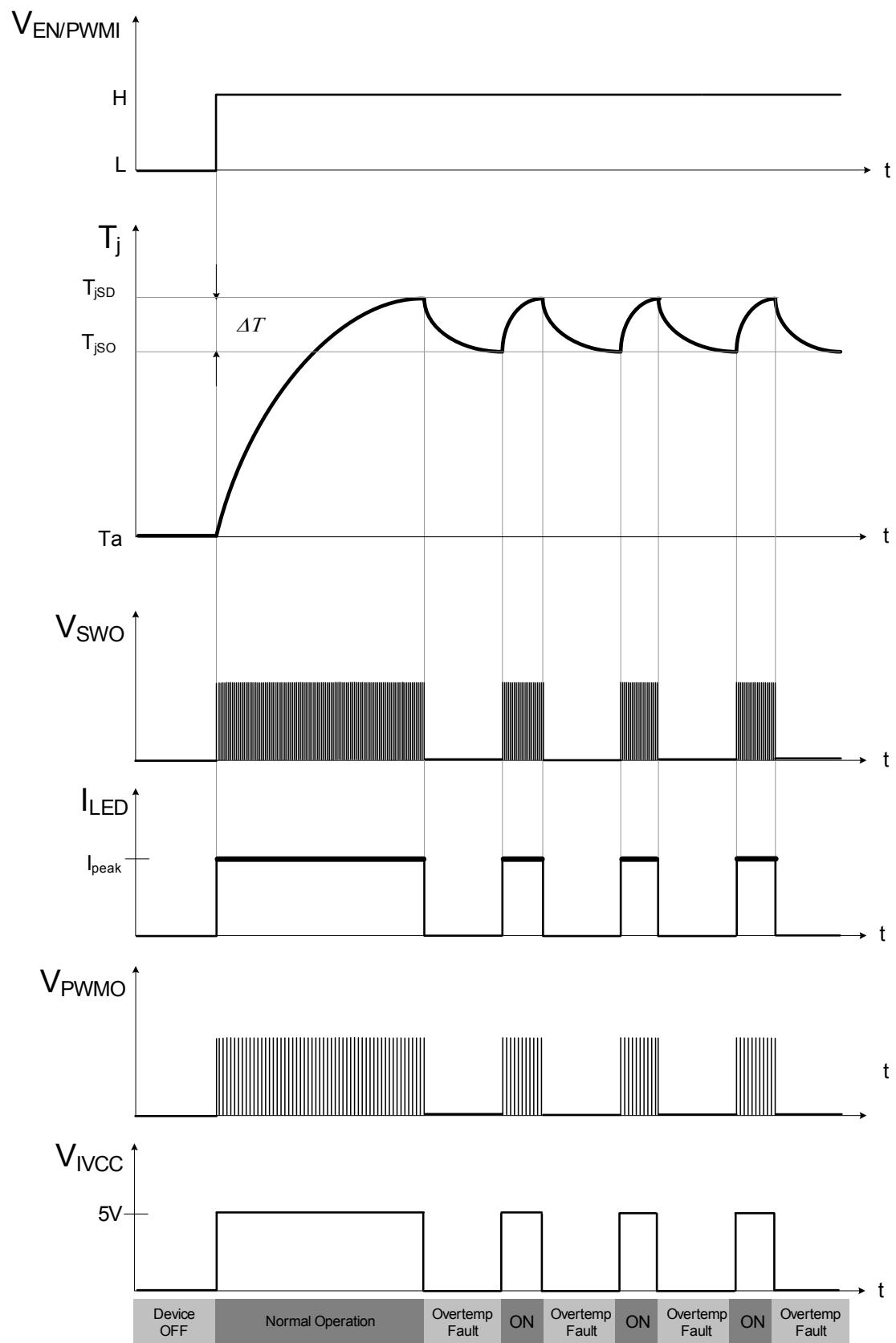
Figure 13 Device overtemperature protection behavior
