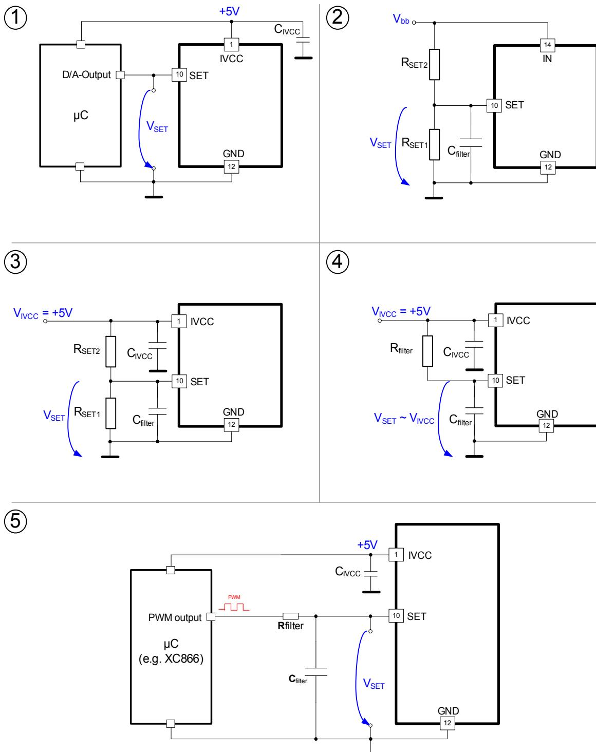
Figure 18 Analog Dimming in various applications
