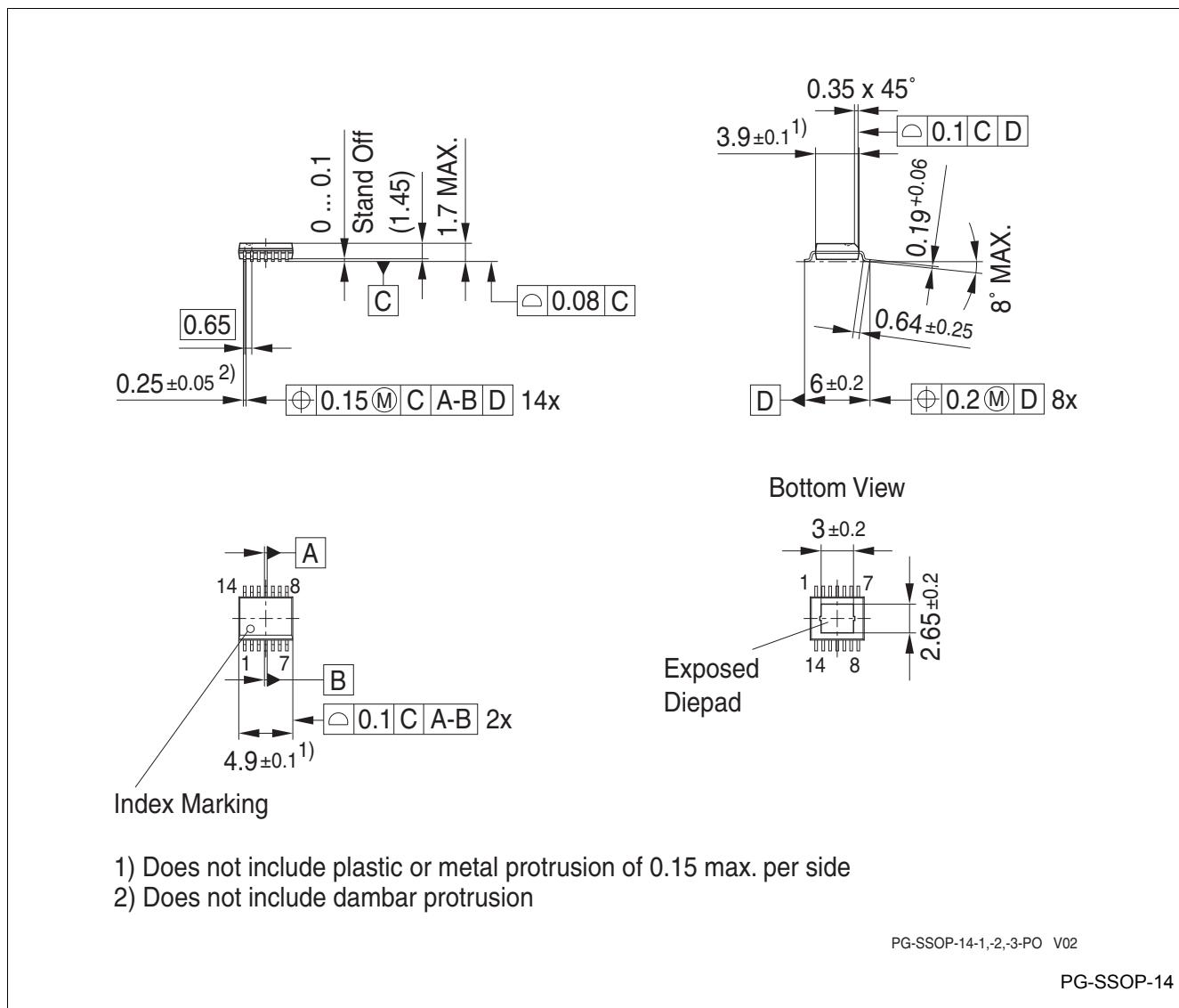
Figure 31 PG-SSOP-14
