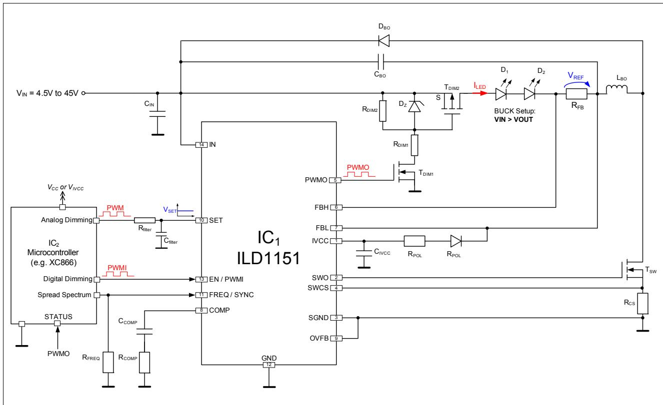
**Figure 27 Buck Application Circuit + Short Circuit protection**
