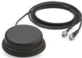
Combined mobile phone GPS antenna with omnidirectional characteristic, 2 m antenna cable with SMA round plug (GSM/UMTS) and R-SMA round plug (GPS)
