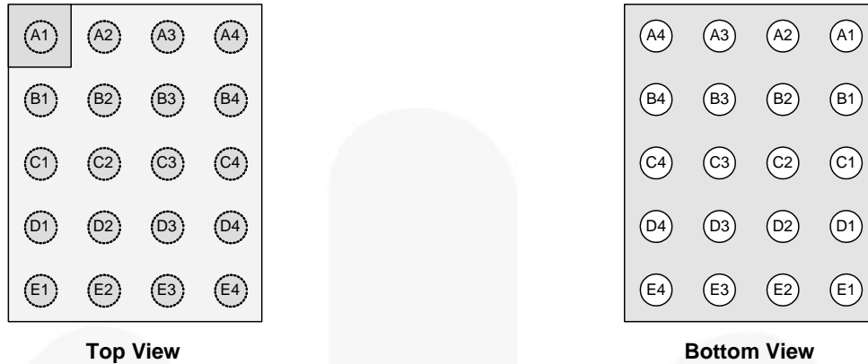
Figure 3. WLCSP-20 Pin Assignments
