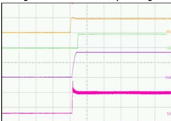
(VIN = 5 V, VOUT = 1.8 V, IOUT = 3 A, no CSS) Upper Trace: Enable Pin Voltage, 5 V / div Second Trace: Power Good Pin Voltage, 5 V / div Third Trace: Output Voltage, 2 V / div Lower Trace: Inductor Current, 2 A / div Time = 2 ms / div
