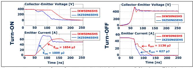
Figure 19 Measured waveforms of an IKW50N65EH5 IGBT during turn-on (left) and turn-off (right) at  $I_c$ =50 A and  $T_c$ =25°C, in both, 4-pin and 3-pin configurations
