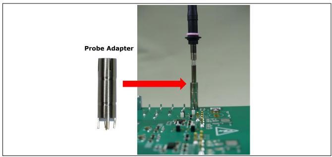
Figure 13 Probe adapter soldered on the Eval board
