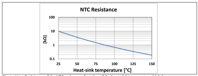
Figure 11 Resistance of the NTC resistor as function of the heat sink temperature (right)
