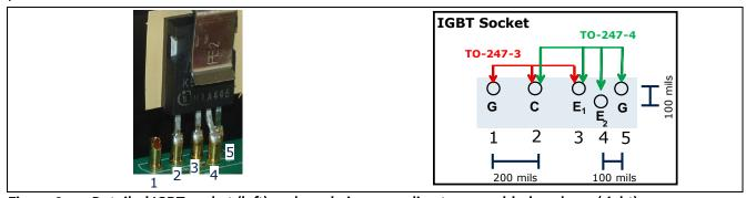
Figure 6 Detailed IGBT socket (left) and used pins according to assembled package (right)
