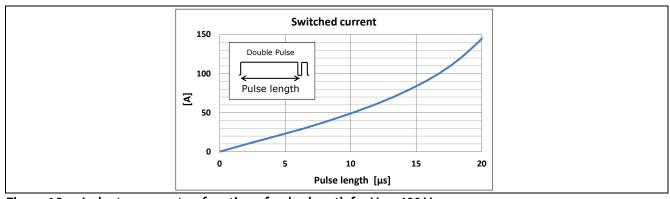
Figure 16 Inductor current as function of pulse length for V<sub>DC</sub> =400 V
