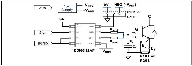
Figure 8 Simplified schematic of the gate driver circuitry
