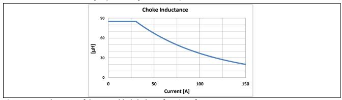
Figure 15 Inductance of the assembled choke as function of current
