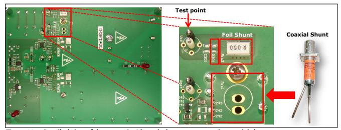
Figure 14 Detailed view of the test point Vic and where to connect the coaxial shunt
