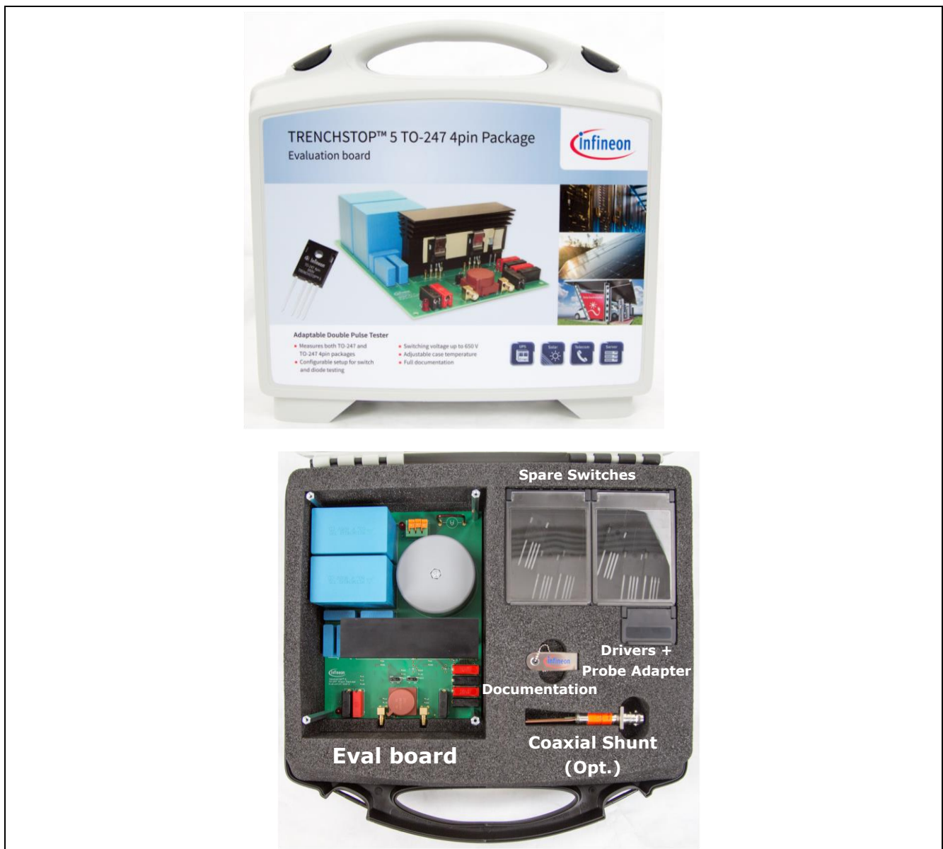
Figure 2 Eval board case and components contained inside
