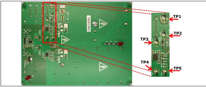
Figure 12 Detailed view of the test points on the back side of the Eval board
