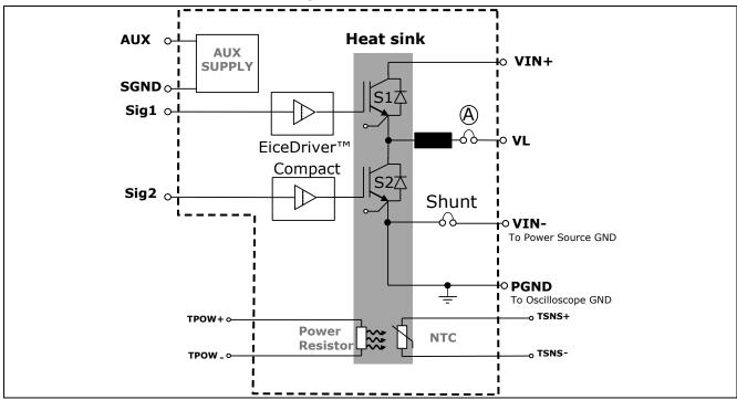
Figure 3 Block diagram of the TO-247 4pin Evaluation Board.
