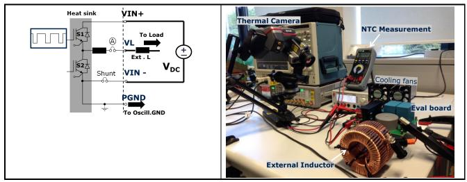
Figure 20 Eval board test bench in Conf. 4
