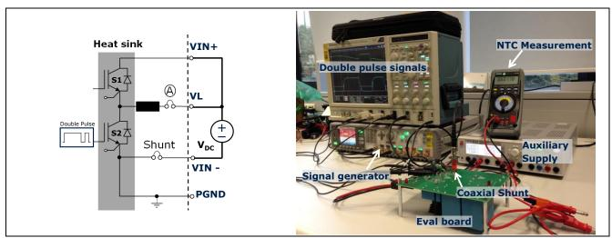
Figure 17 Eval board test bench in Conf. 2
