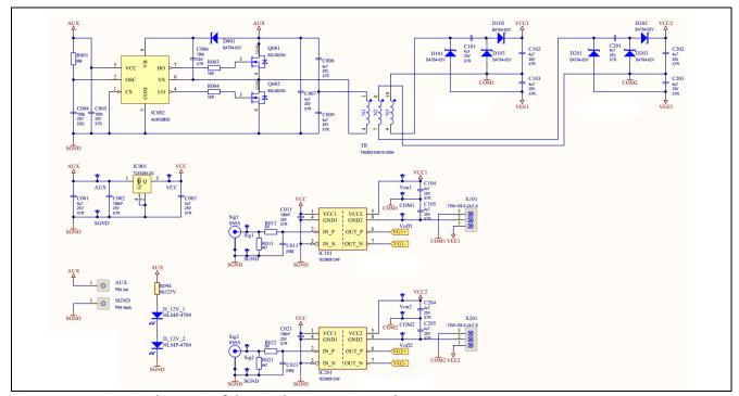
Figure 23 Circuit schematic of the auxiliary power supply
