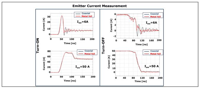
Figure 18 Measured waveforms of the emitter current of an IKW50N65EH5 IGBT. Turn-on events are depicted on the left side, turn-off on the right side, using both coaxial and metal foil shunts, for different current values
