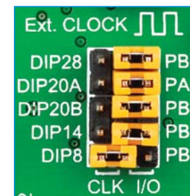
Figure 4-10: Position of the jumpers for DIP8
