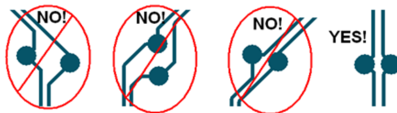
Figure 13 • Example of Asymmetric and Symmetric Differential Pairs Structure
