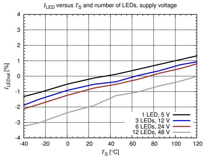
**LED current vs. soldering point temperature:**  $R_{\text{sense}} = 178 \text{ m}\Omega$ ,  $L = 68 \mu\text{H}$ ,  $V_{\text{fLED}} = 3 \text{ V}$ ,  $R_{\text{Tadj}} = 0 \Omega$ .
