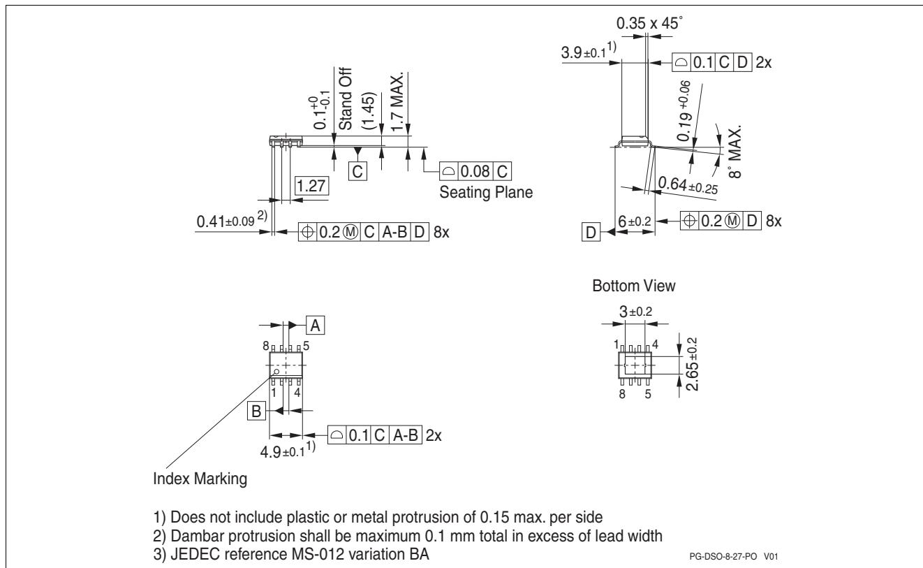
**Figure 9 Package outline PG-DSO-8-27 (dimensions in mm)**
