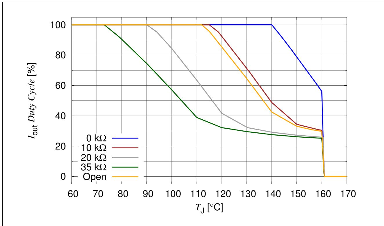
**Figure 3** Typical Output Current Duty Cycle of Over-Temperature Protection vs. T<sub>J</sub> and R<sub>Tadj</sub>
