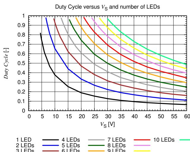
**Performance vs. supply voltage and number of LEDs:**  $R_{\text{sense}} = 353 \text{ m}\Omega$ ,  $L = 150 \mu\text{H}$ ,  $V_{f,\text{LED}} = 3 \text{ V}$
