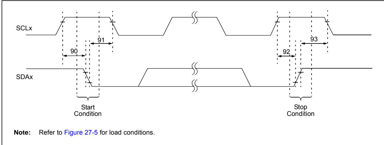
**TABLE 27-35: I<sup>2</sup>C™ BUS START/STOP BITS REQUIREMENTS (MASTER MODE)**
