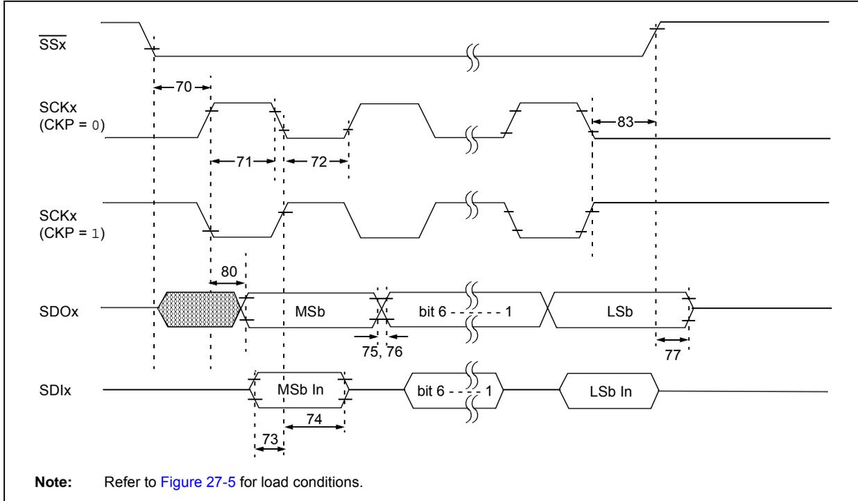
**TABLE 27-31: EXAMPLE SPI MODE REQUIREMENTS (SLAVE MODE TIMING, CKE = 0)**
