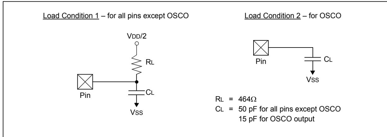
**TABLE 27-19: CAPACITIVE LOADING REQUIREMENTS ON OUTPUT PINS**
