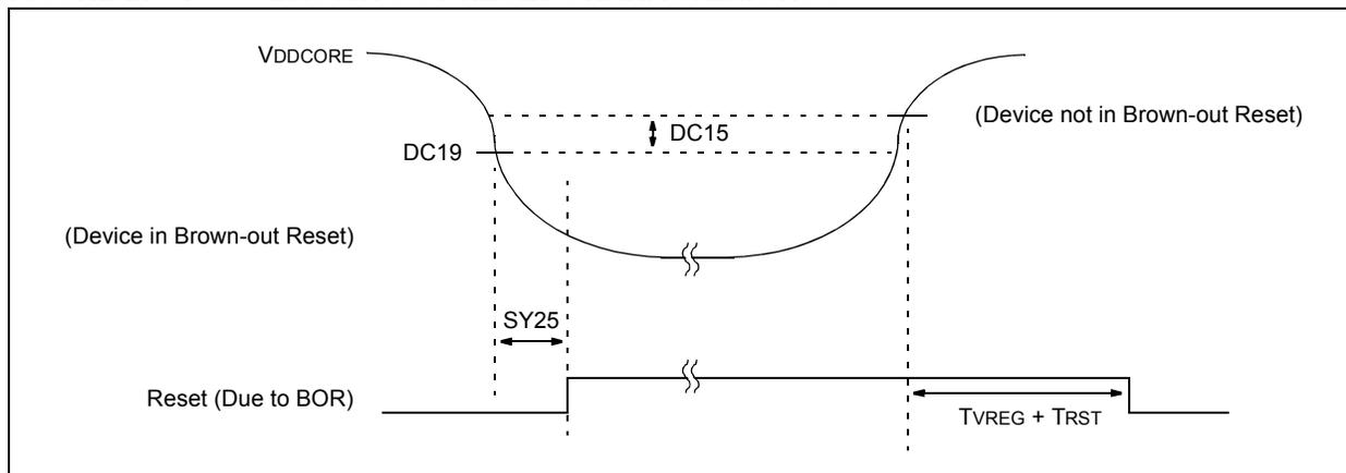
**TABLE 27-25: RESET, WATCHDOG TIMER, OSCILLATOR START-UP TIMER, POWER-UP TIMER AND BROWN-OUT RESET TIMING REQUIREMENTS**
