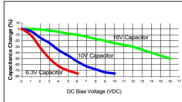
When selecting a ceramic capacitor to be used with the internal voltage regulator, it is suggested to select a high-voltage rating, so that the operating voltage is a small percentage of the maximum rated capacitor voltage. For example, choose a ceramic capacitor rated at 16V for the 3.3V or 2.5V core voltage. Suggested capacitors are shown in [Table 2-1](#).
