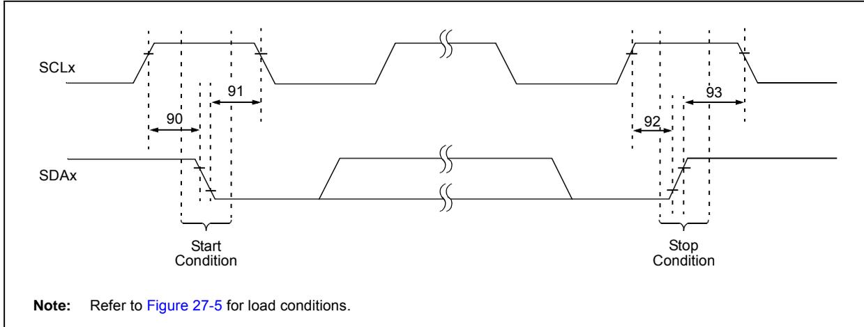
**TABLE 27-33: I<sup>2</sup>C™ BUS START/STOP BITS REQUIREMENTS (SLAVE MODE)**
