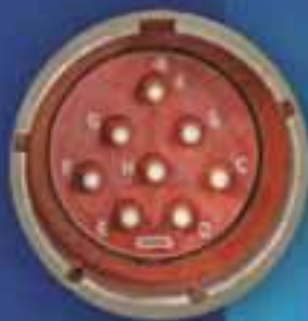
MIL-PRF-29504 Size 16 Fiber Optic Termini
