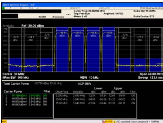
Figure 30. AD9135 Four-Carrier W-CDMA ACLR, f_{OUT} = 30 MHz, f_{DAC} = 1966 MHz, 4\times Interpolation, PLL Frequency = 245 MHz
