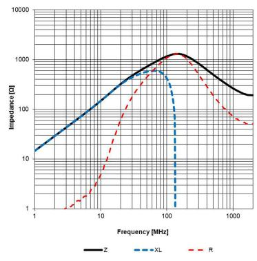
Test Equipment: E4991A or equivalent
